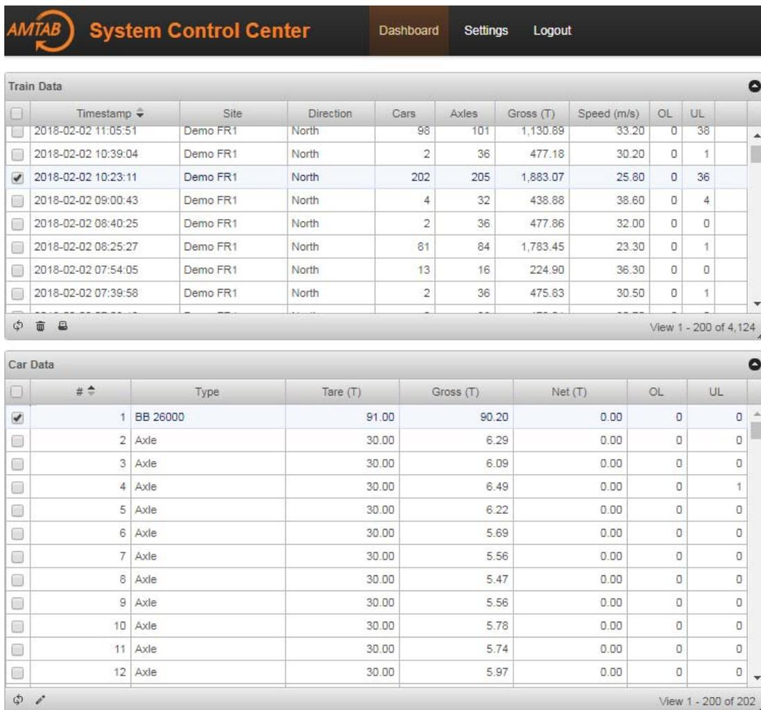
The screenshot displays the AMTAB System Control Center interface. At the top, there is a navigation bar with the AMTAB logo and the text "System Control Center", along with menu items for "Dashboard", "Settings", and "Logout". Below this, there are two data tables.
